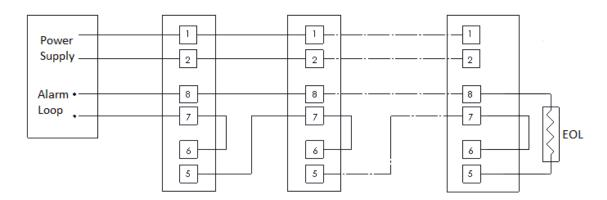
FIGURE 19 - 4 WIRE RELAY CONNECTION
