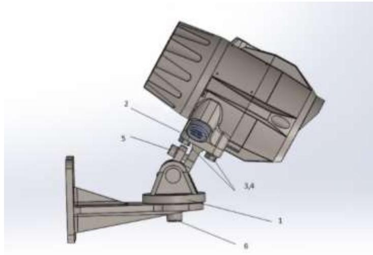
**FIGURE 13 - DETECTOR ON TILT MOUNT – SIDE VIEW**
