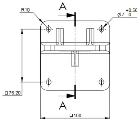
**Figure 11: Tilt Mount Base - Plate View**
