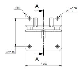
Figure 11: Tilt Mount Base - Plate View
