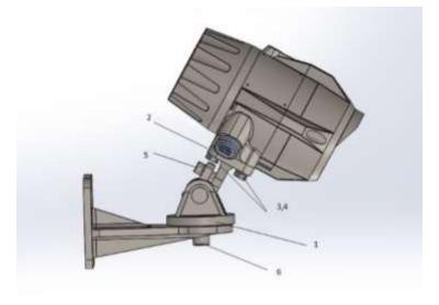
FIGURE 13 - DETECTOR ON TILT MOUNT - SIDE VIEW
