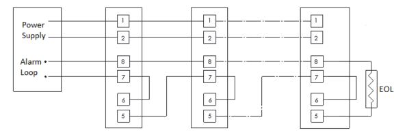
FIGURE 19 - 4 WIRE RELAY CONNECTION
