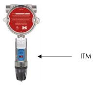
The latest version of the DM700 and PI700 ITM's include both a black 0V electrical ground connection as well as a striped green/yellow earth ground connection. Section 2 of the manuals for these two products has always noted that:
