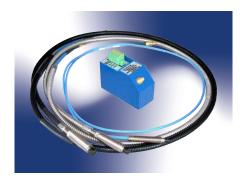
The FK-202F transducer is eddy current type non-contact displacement/vibration transducer, used for measuring Shaft Vibration, Axial Position, Rotating Speed and Phase Mark (Phase Reference) from small rotating machinery to large critical machinery such as turbines and compressors in plants.
