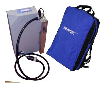
The Procal 9000 range of portable gas / water vapour blenders are designed to carry out field testing and recalibration of installed Continuous Emission Monitoring Systems (CEM) / Automated Measuring Systems (AMS) safely and securely. Designed for ease of use in the industrial environment, they are mounted in a customised backpack to enable safe use when accessing elevated platforms.
