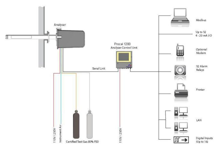
The Control Unit can support multiple analysers from the Procal range
