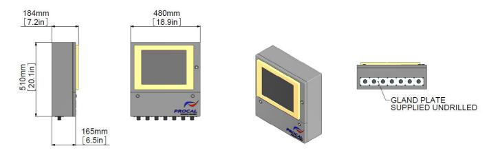
This unit has been specifically designed to be located in "On Plant" environments where conditions are not be conducive to the use of a typical office PC.
